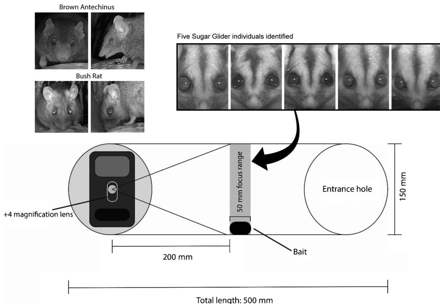
**Figure 1.** Selfie trap design: a 150 mm diameter white PVC pipe, with a camera fixed to a PVC pipe cap facing a bait station. A close focus lens is fixed on the camera lens, allowing focused images to be captured between 200–250 mm from the front of the camera. Five individual Sugar Gliders identified from a single selfie trap are shown. Example side and front photos of Brown Antechinus and Bush Rat are shown.
