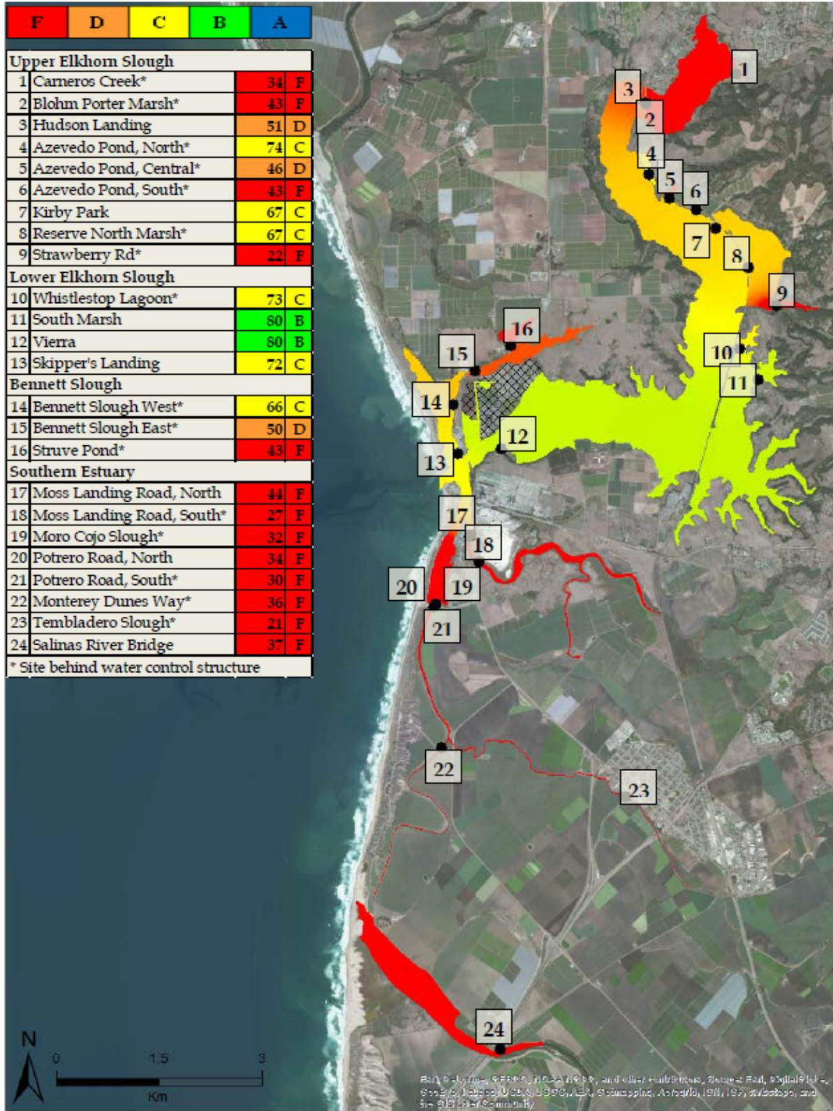
Figure 2-3. Resultant grades and spatial interpolation of index values calculated using the WQI approach. Source: Mercado et al. 2014
