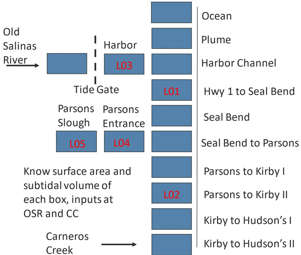
Figure 3-14. Schematic of Box Model of Elkhorn Slough with LOBO Mooring Locations (Figure courtesy of Ken Johnson)
