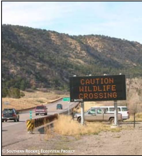
VARIABLE MESSAGE SIGN ON US HIGHWAY 550, NORTH OF RIDGWAY, COLORADO.
