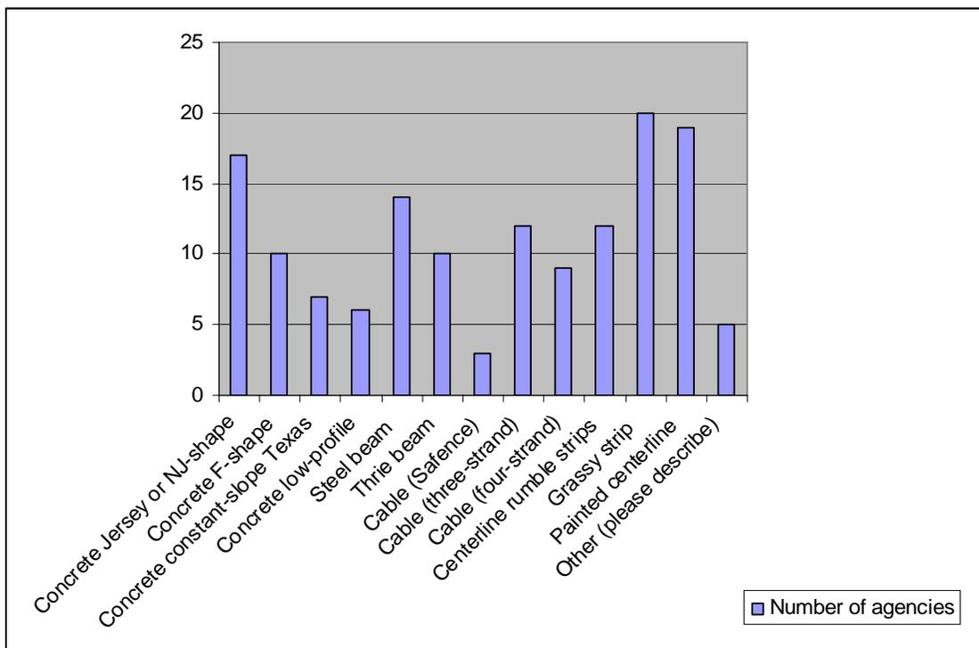
Figure 6. Agency use of different median barrier types.
