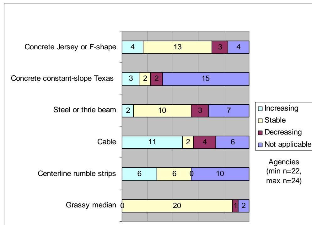
**Figure 23. Comparison of median barrier installation trends by type.**
