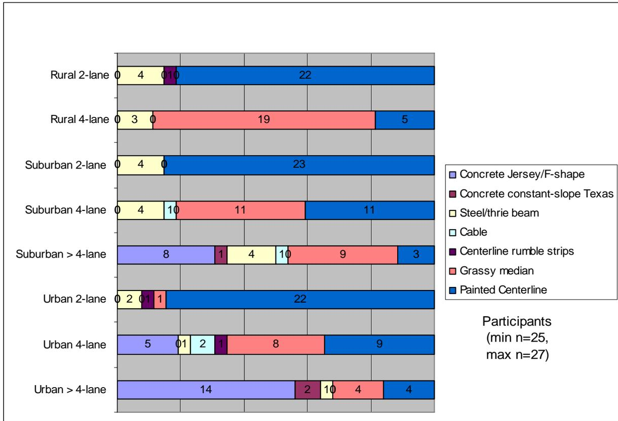
Figure 24. Median barrier types used by roadway type.
